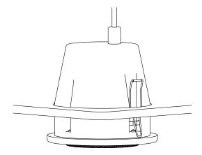
3) When the speaker is mounted, push both springs downwards to lock the speaker in in place. Once the springs are pushed down, the speaker will place itself properly in line with the panel. In this image the AWP06 speaker is locked tightly and ready for use.
