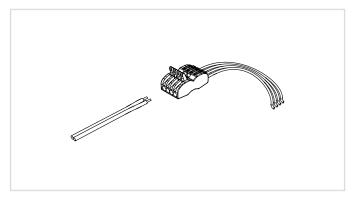
Connect the wires coming from the amplifier to the SnapConnect™ on the rear speaker part.
