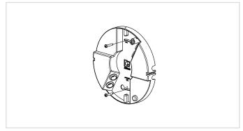
The wall part has to be assembled to the provided location on the wall or ceiling. This is done through knocking out the provided areas (teardrop holes) for the fasteners. Choose the fasteners depending on the mounting surface (concrete, wooden, steel, ...) The distance between both mounting positions is 130 mm.
