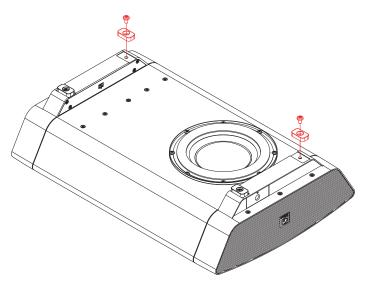
Step 2: Assembling the cabinet supporting bar
