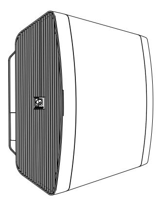
The aluminum enclosure features a grill on both sides, whereof one side includes the bass port. To allow optimal air-circulation through the bass port, make sure this side remains uncovered when installed.
