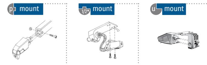
A P-mount cartridge has four terminals at the back that simply plug in to the end of the tone arm. The cartridge is then secured to the tone arm with a single screw.
