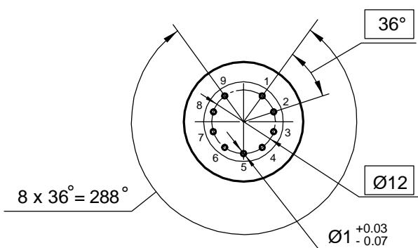
Electrode -to - lead connection diagram
