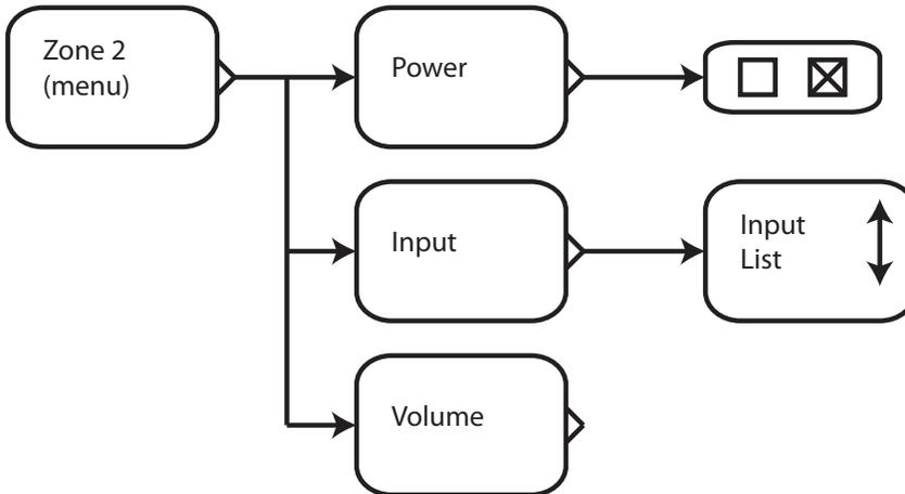
The **Zone 2 Menu** contains the settings and controls typically used to control the second audio zone in the day-to-day operation of your RMC-1. These are settings that are typically chosen each time when viewing content.
