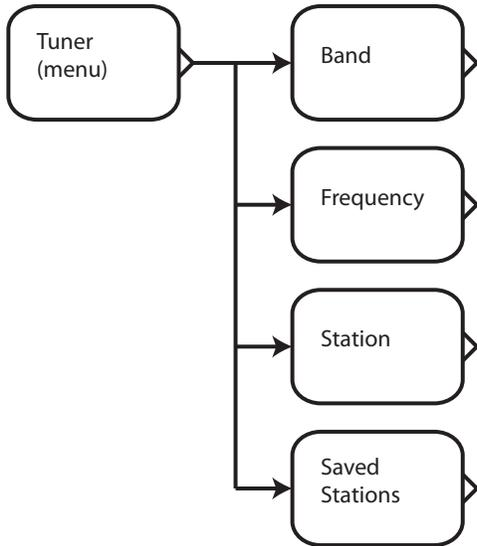
The **Tuner Menu** is used to select a station on the RMC-1's built-in high quality AM/FM tuner, and to create, rename, and delete station presets.
