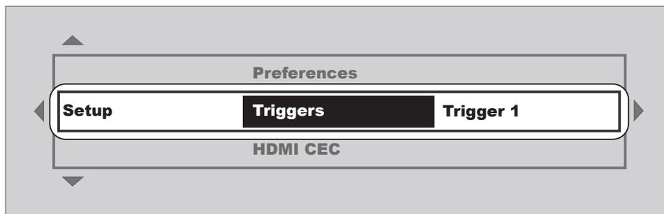
The small arrows to the left, right, above, and below show you which directions you can move in the menu from your current location. Highlight LEDs will also illuminate in the halo ring around the front panel encoder knob to indicate valid directions for movement within the menu.
