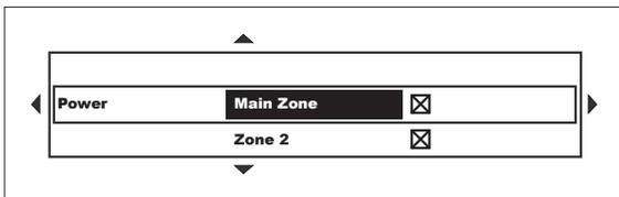
As you can see, we're in the final menu screen for configuring how Trigger 1 will respond to Power conditions. All we have to do is use the Up and Down arrow buttons to select Main Zone, and then Zone 2. Then, for each of those, use the Right arrow button to move to the check box, the Up and Down arrow buttons to check the box, and the Left arrow button to move back to where we are. After we've checked the box for both zones, we'll use the Menu button to exit back to the Information screen.
