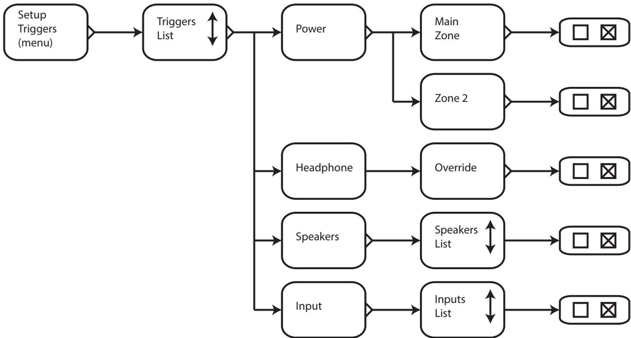
The **Setup Triggers Menu** allows you to configure how the triggers on the RMC-1 operate.
