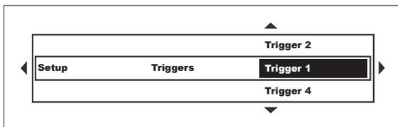
Since we want to configure one of the Triggers, use the Up, Down, and Right arrow buttons to select the particular Trigger we want. At this point the arrows show that we can move up or down to select the Trigger we want to configure. Since Trigger 1 is already the active choice, use the Right arrow button to select it and enter into the Trigger 1 section of the Setup Triggers Menu.
