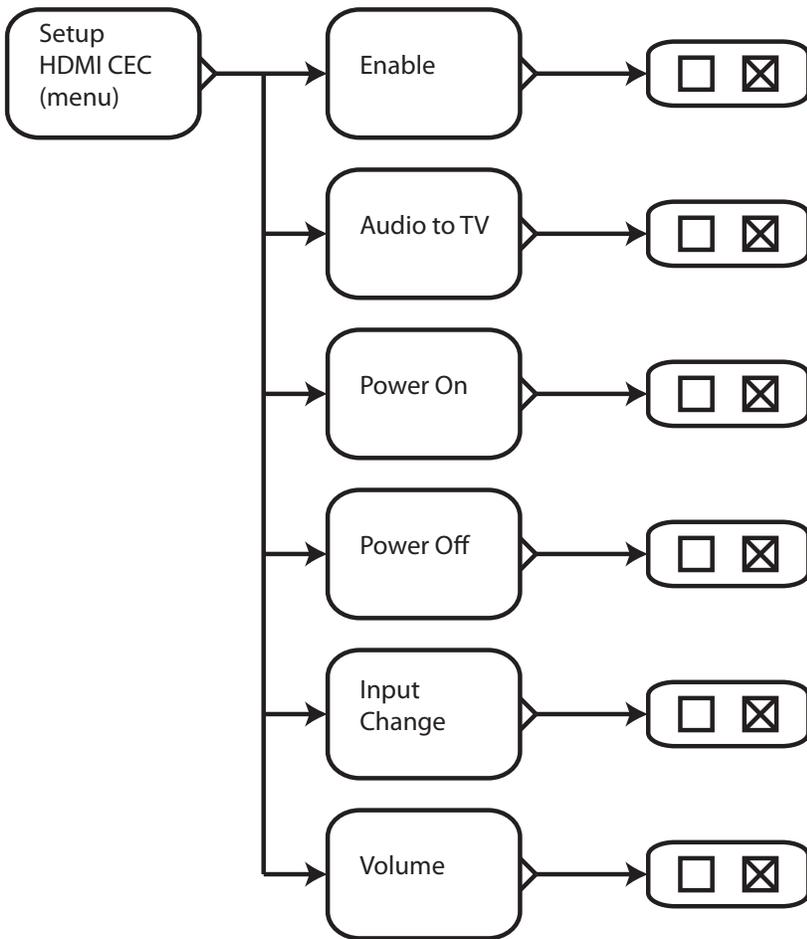
The **Setup HDMI CEC Menu** allows you to configure what types of CEC commands the RMC-1 sends and responds to.
