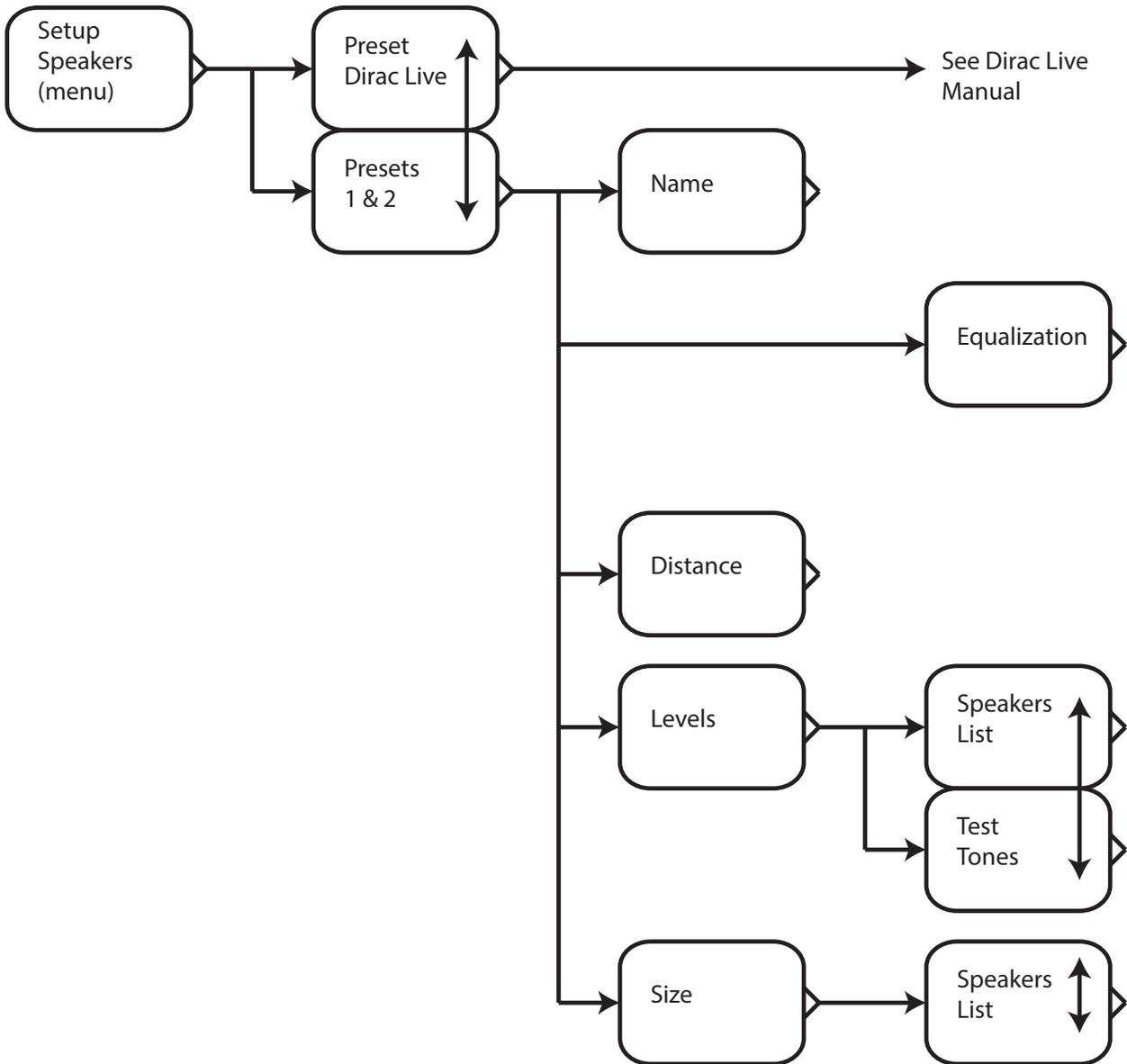
The **Setup Speakers Menu** is where you access the powerful speaker and room correction features of the RMC-1, including Dirac Live automatic room correction, and the RMC-1's incredibly flexible manual calibration system, which includes two fully independent banks of parametric equalizers, along with pink noise and test tone generators.
