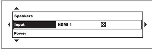
This time the highlight is showing us that the active choice is to configure how Trigger 1 responds to each Input. Since this time the default choice is not the one we want, use the Down arrow button to move to Power, which is the option we want.
