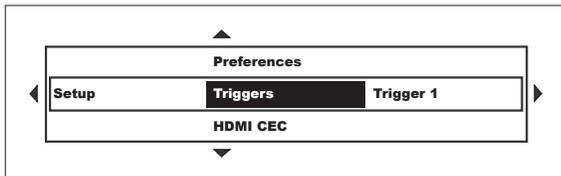
Press the Right arrow button to enter the Setup Menu. Now the highlight shows that the active choice is Triggers, and we can move up to the Setup Preferences Menu or down to the Setup Network Menu. Use the Right arrow button to move to the Setup Triggers Menu.
