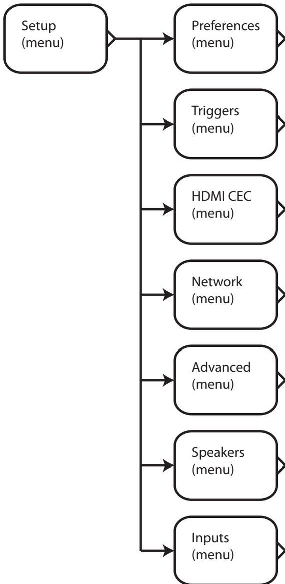
The **Setup Menu** allows you to view and change the main configuration settings for the RMC-1.
