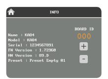
The Info page contains information about the current software and firmware, and the Board ID of the amplifier. When connecting the amplifier in a K-framework network, please make sure that all devices in the network have different ID numbers.
