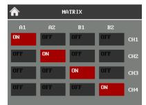
The Matrix page allow users to manage the routing of the four input channels to the four output channels.
