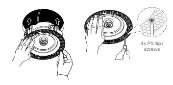
**6** Reposition the grill on the loudspeaker.
