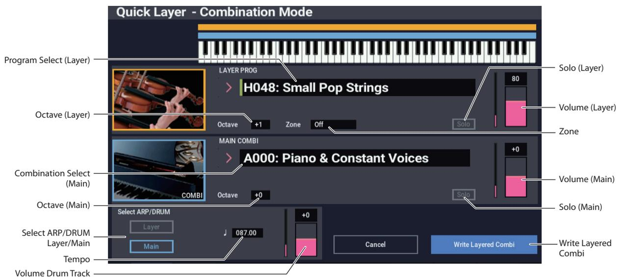
Here, we’ll walk through a typical use of Quick Layer: adding a string layer to a piano sound. Many of the steps are identical to the Quick Layer functionality in PROGRAM mode, but there are a few differences unique to COMBINATION mode. Let’s start with the piano:
