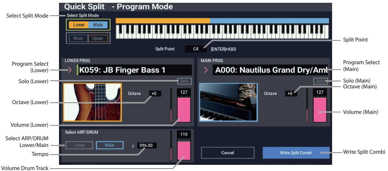
Quick Split makes it easy to create common setups, such as piano for the right hand and bass below for the left, or electric piano for the left hand and a lead synth for the right. Let's walk through the first example: a bass and piano split.
