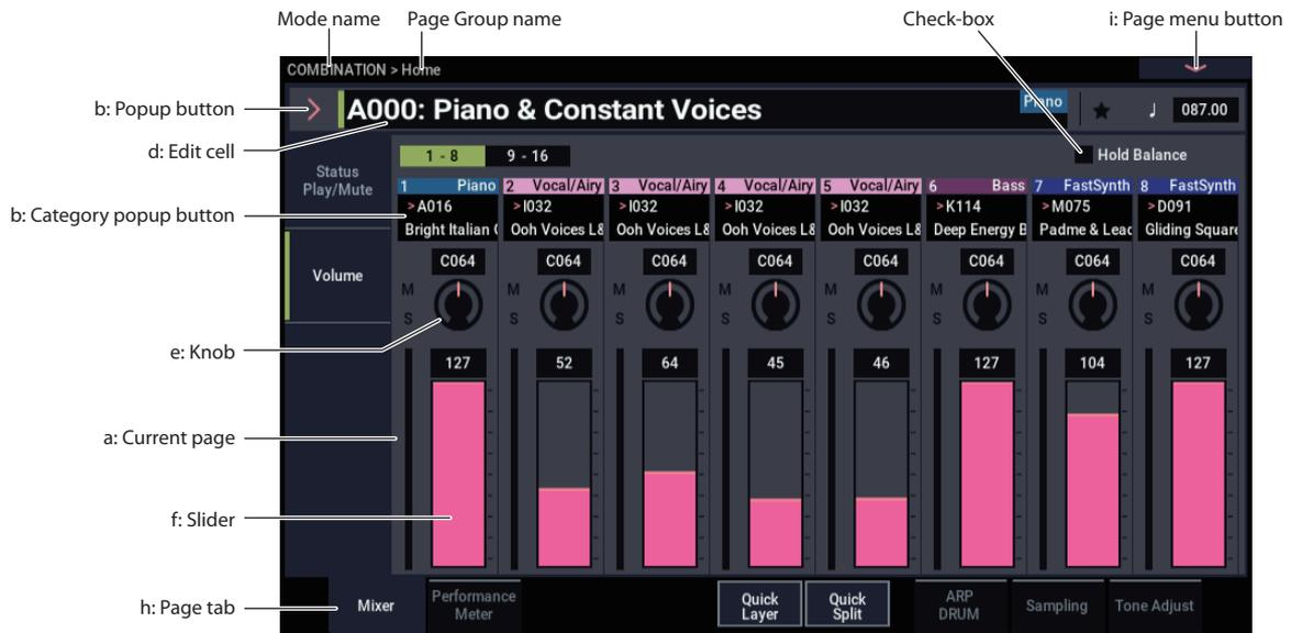
The NAUTILUS uses Korg’s TouchView graphical user interface. By touching objects displayed in the LCD screen, you can select pages, set parameter values, move sliders and knobs, enter text, connect virtual patch cables, and more.
