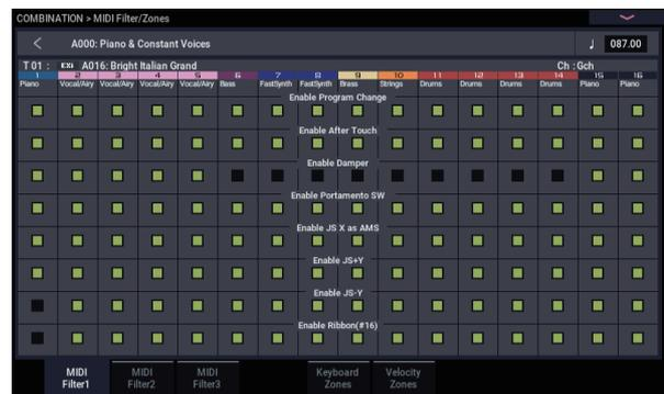
The MIDI filters don't turn the functions themselves on or off. Instead, the filter just controls whether or not that MIDI message will be transmitted and received.
