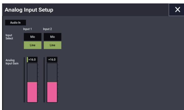
Choose the Mic setting only when connecting a mic. Note that some microphones, such as condensers, may require external phantom power, which is not supplied by the NAUTILUS.
