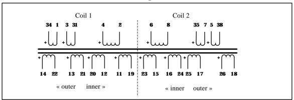
LL1620CFB Primary connection for push-pull output stage with 25% cathode feedback
