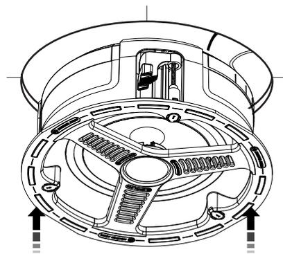
**5** Tighten the 3 Tri-Grip screws and replace the protective screw covers.
