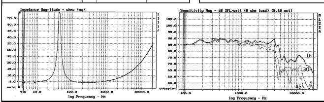
Measured on IEC baffle using Bruel & Kjaer 3144 model microphone.
