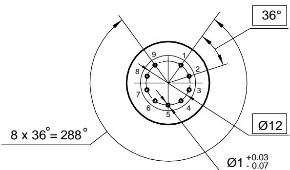
Electrode -to - lead connection diagram
