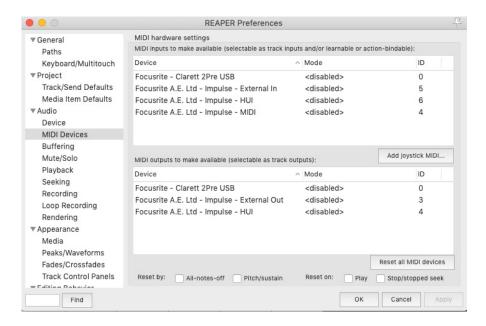
Navigate to the 'Control/OSC/web' tab in the 'Reaper Preferences' window and click 'Add' to add a new control surface. Now, in the 'Control Surface Settings' window, set the Control surface mode to HUI (partial) and set the input and output port to 'Focusrite A.E. Ltd. - Impulse HUI' as shown below.
