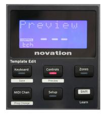
Preview mode is provided to confirm how a control is currently configured without actually transmitting any MIDI data to your computer or elsewhere. Enter Preview mode by holding down **Shift** and pressing the **Controls** button. The LED in the **Controls** button blinks to confirm the mode. Pressing or moving any of the assignable controls will display its MIDI message type. Pressing the **Controls** button again will exit Preview mode.
