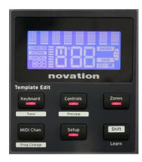
The upper 8-character row of the display shows the Impulse parameter or setting being adjusted. The 3 large characters in the lower row show the parameter value or setting itself. In any of the menus, you can scroll through the available pages with the + and – buttons.
