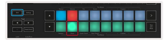
If a Drum Rack is loaded onto the selected Live track, and your Launchkey is in Drum mode, the pads light up the colour of the track. When played the pads will light up green. These pads will play whatever Drum Rack pads are visible on your computer screen. Pressing the ▲ ▼ buttons scrolls up/ down through a Drum Rack's bank of 128 pads, each press moves up or down the rack in banks of 16.
