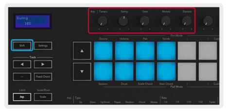
**Tempo** – This knob speeds up or slows down your arpeggio relative to the Arp Rate. When Launchkey is used as a standalone controller, this knob ranges from 60 BPM to 187 BPM. However, when synced with Ableton Live, this knob will have no effect.
