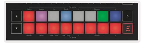
**Solo (Blue)** - Pressing the pads will solo the corresponding tracks, meaning only tracks with Solo on will be heard. The pads dimly glow if tracks are not soloed (i.e. they are silent). Soloed tracks glow a steady bright blue.
