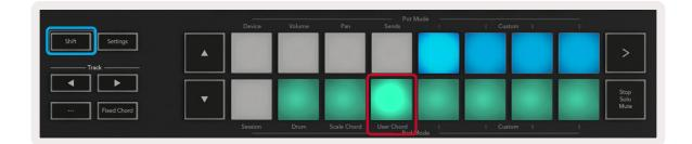
To assign a chord to a pad simply press and hold the pad and press the notes that you want to assign from the keyboard. Up to 6 notes can be assigned to each pad and can be input with individual pushes of the keys, meaning you do not need to hold down all the notes at once so long as the pad is being held.
