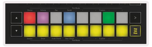
**Clips (Multi**) – the fourth press (after toggling through Stop, Solo and Mute) changes the function of bottom pads back to the default Session mode, where the bottom row of pads will again represent clips.
