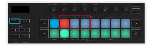
**2.3.1.1 Volume** - This mode allows you to control Track Volumes using the pots. To select this mode, hold the Shift button and press the Volume pad.
