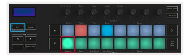
**Record/ Mute mode** - the top row of pads toggles the record arm on the relevant track and will be lit red, the bottom row toggles the track mute and will be lit yellow. The tracks represented by the pads include any sends tracks, the top row of pads will not be lit for sends (buses).
