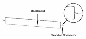
Secure the backboard to the sideboards with 4 M5\* 35 screws.
