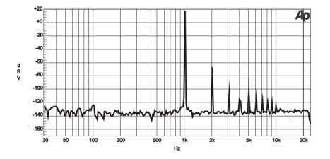
Distortion spectrum of line stage, 5 V output at 1 kHz. The low level of harmonic distortion and low noise level are clearly visible. There are no hum components at 50 Hz and 100 Hz.
