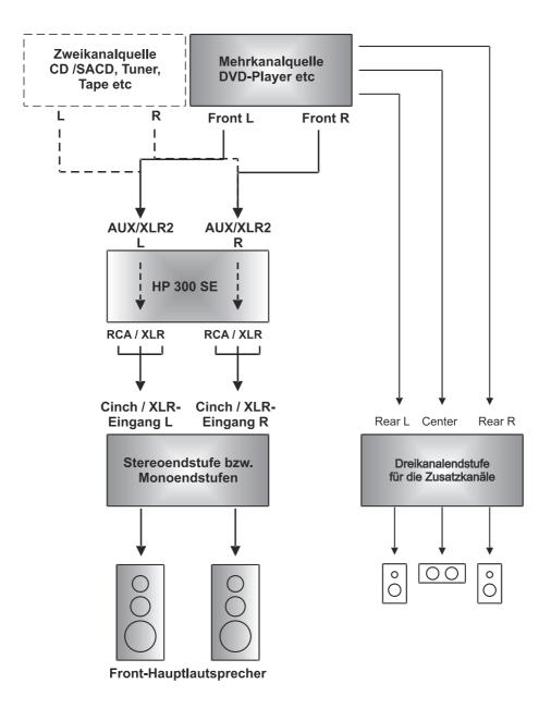
In the multi-channel mode the volume of the multi-channel system has to be adjusted at the multichannel source, eg the DVD player, TV, etc. In the bypass mode the volume control of the HP300SE is out of function.
