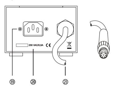
Mains Input, IEC receptacle Serial number and mains voltage Connecting cable with plug connector
