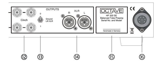
RCA Outputs for unbalanced Power Amplifiers Double Output to allow BI - Amping
