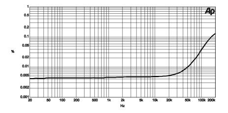
Overall distortion (THD + noise) of the line stage from 20 Hz to 200 kHz. Distortion remains low up to 20 kHz
