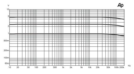
Frequency response accuracy of line stages in 'Gain Low, Med and High. In the frequency response of 20 Hz - 200 kH.
