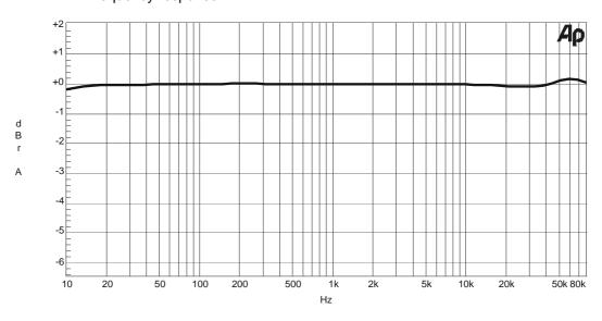
Between 10 Hz and 90 kHz the frequency response tolerance is within 0.3dB
