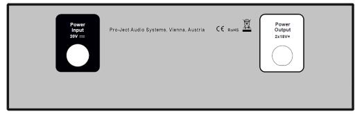
Connect the Power Box RS Phono with Phono Box RS with supplied cable. Then connect supplied power supply to the Power Input 20V DC socket and to the mains. The original power supply of Phono Box RS is no longer required.
