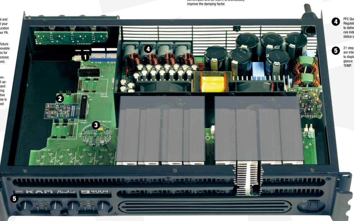
Newly designed short tunnel cooling system forces air directly onto the high efficiency heat-sinks and the o/p devices bolted directly to them. PFC QuantaPulse<sup>™</sup> Regulated Dual SMPS front end to deliver their full performances independently of mains status or load requirements.
