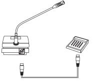
Connection: connect the microphone output jack to other equipment like amplifier or mixer. (Picture 5)
