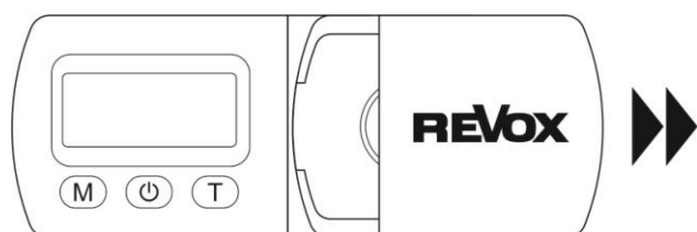
Fig. : Remove protective cover from tonearm scale
