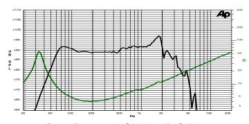
Frequency Response on 35 Lt @ 60 Hz Vented Box @ 1W, 1m Free Air Impedance
