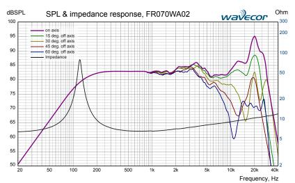
Measuring conditions, impedance Driver mounting: Free air, no baffle, back side open (no cabinet) Input signal: Semi-current-drive, nominal current 2 mA Smoothing: None
